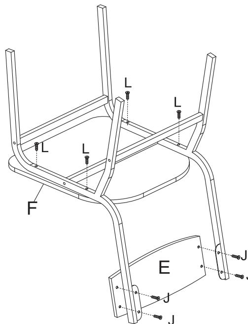
**3** step 3-Use screws(Part L)to connect chair feet(Part G/H)and cross-bars(Part I)as a metal chair frame
